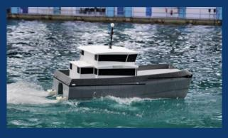
Scale model seakeeping tests have demonstrated the performance and maneuverability of the vessel in a range of different sea states.
