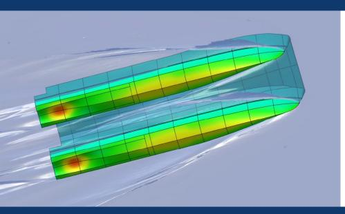
Independent CFD testing has provided validation of the Chartwell hydrodynamic and aerodynamic resistance throughout the speed range.
